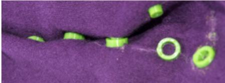
Figure 8. 3D Printed snaps printed onto a fabric.
